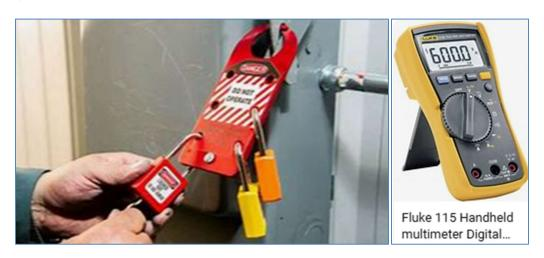
**When** – Where work is to be undertaken on plant or a specific area of equipment of the plant and power is not required, the plant must be completely de-energised (brought to 'zero energy state') and locked and tagged out from its power source.
